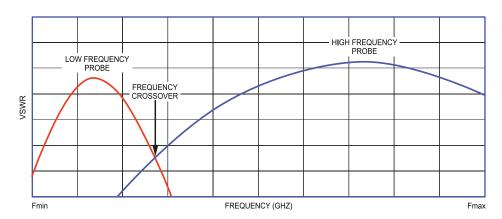
VSWR versus Frequency of a two-probe slide-screw tuner.
